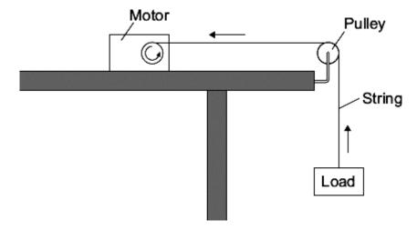
In the motor, the electrical energy is transferred into other types of energy. Some of this energy is useful and the rest of the energy is wasted.
